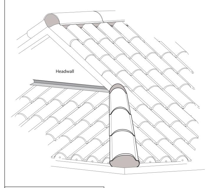
Hip installation is the same as Ridge installation. See pages 14 through 16 of this manual for details and information on fastener size, type and location.
